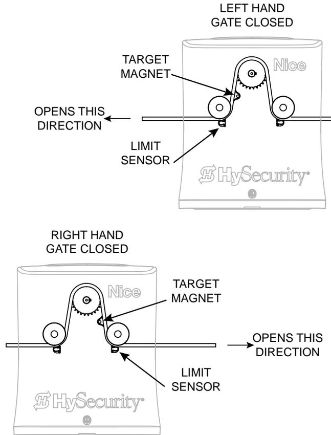
Figure 19. Limit Sensor and Target Magnet Position
