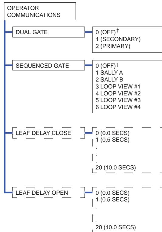
LEAF DELAY OPEN/CLOSE ONLY APPEAR IF THE GATE OPERATOR IS SET UP AS PRIMARY OR SECONDARY.
