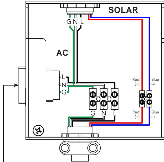
Connect service outlet lead wires to 115VAC only.
