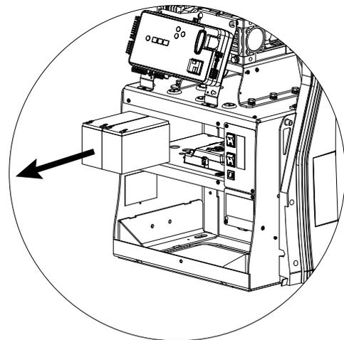
Figure 48. Remove the Batteries
