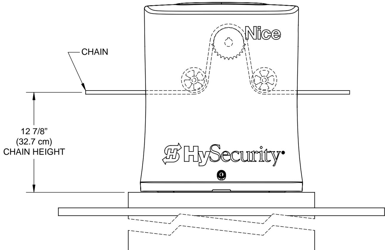
Figure 5. Front Installation Chain Height
