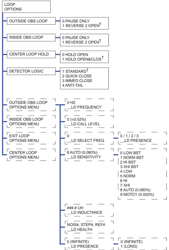
MENU STRUCTURES FOR LOOP OPTIONS ARE VISIBLE AND CONFIGURABLE ONLY WHEN AN HY5B MODULE IS INSTALLED INTO THE SMARTCNX CONTROLLER. OOLD, IOLD, ELD, AND CLD SUB-MENUS ARE IDENTICAL.
