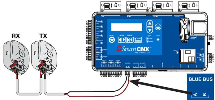
NOTE: Matching wire polarity is not required for BlueBUS photocells.
