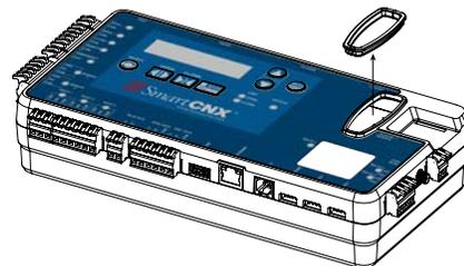
Figure 41. Remove OXI Port Rubber Plug
