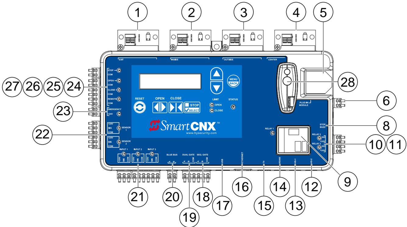
Figure 31. SmartCNX Controller Connections
