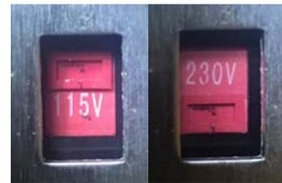
Figure 25. Voltage Switch Positions
