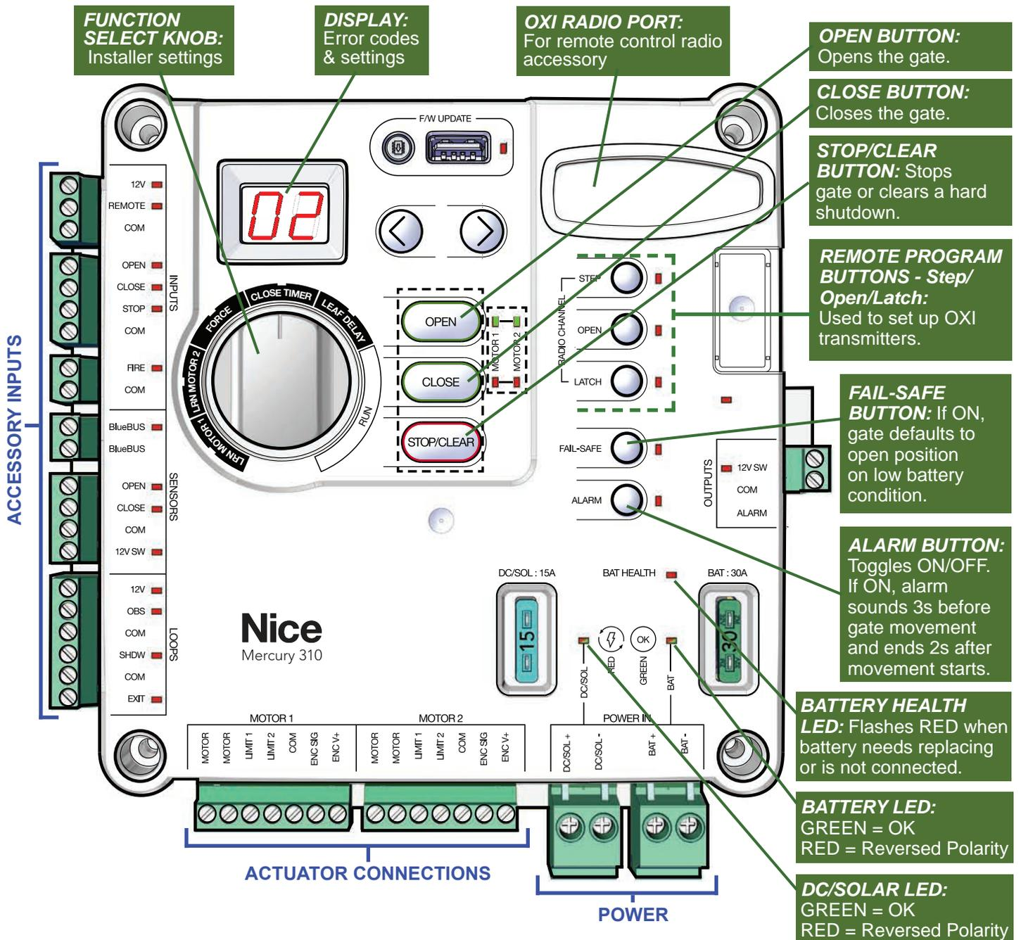
FIGURE 3: Mercury 310 Control Board Interface Features
