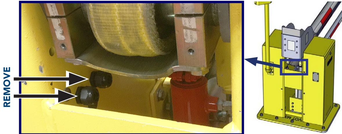
IMAGE 11-1: REMOVE EXISTING CORD GRIPS
