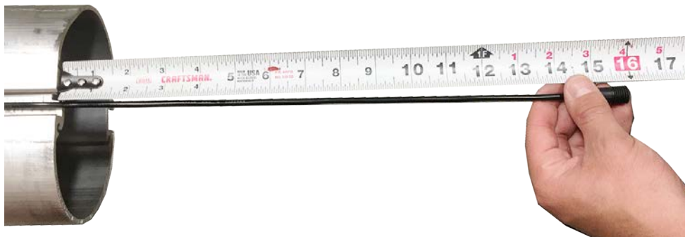
IMAGE 6-6: CABLE AT 16" LENGTH FROM END OF ARM
