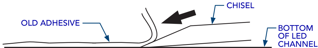
IMAGE 5-1: CHISEL SCRAPING OFF OLD ADHESIVE (SIDE VIEW)
