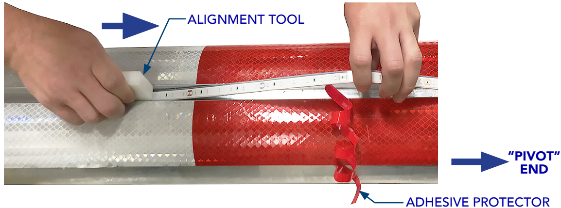
IMAGE 6-4: USING THE LED STRIP ALIGNMENT TOOL
