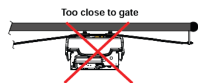
Figure 18. Incorrect Distance to Gate
