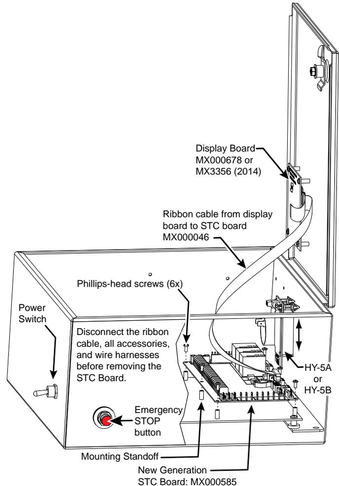
Figure 3. Control Box - Cut-away view of the SDC Board in a SwingSmart DC Operator
