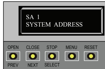
**2** Press Select again to set gate operator's system address (Each gate operator attached to the same HyNet must have a unique SA number. Choose 1, 2, 3, or 4.)
