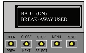
Program Breakaway switch, if needed
