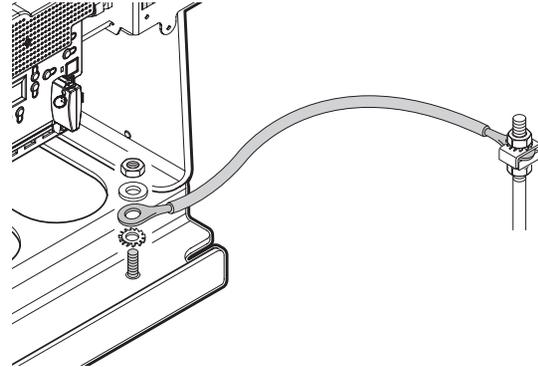
Figure 19 - GROUNDING WIRE
