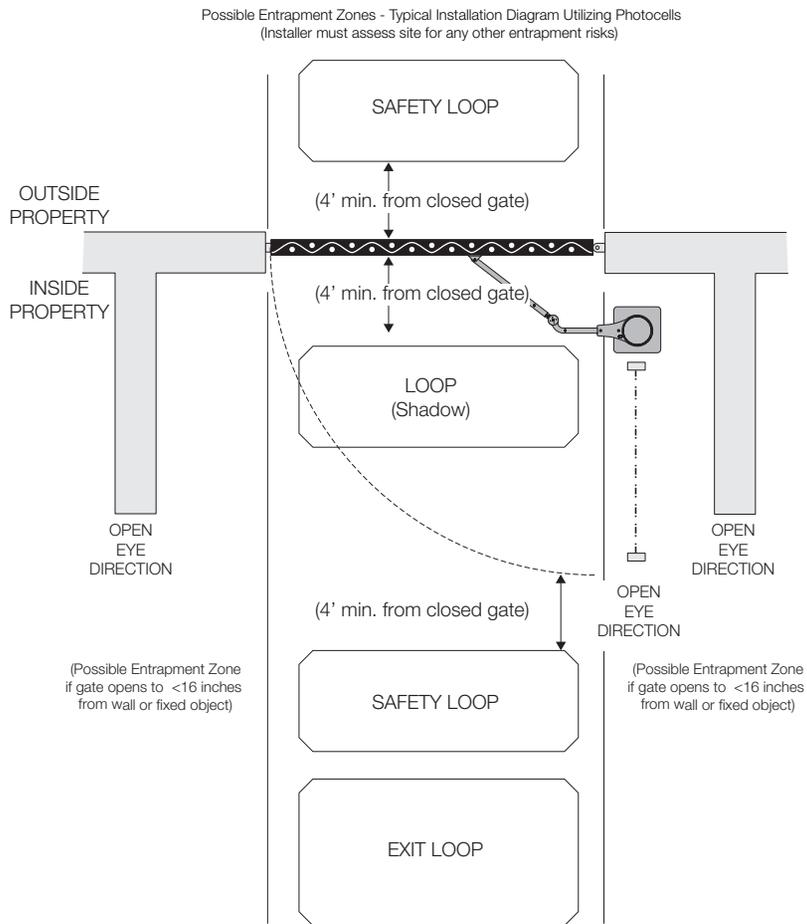
Figure 26 - GENERAL GATE LAYOUT IN-GROUND LOOPS
