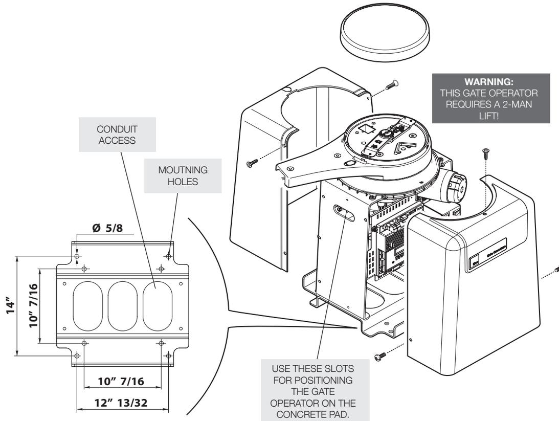
Figure 1 - SWING OPERATOR CUT-AWAY
