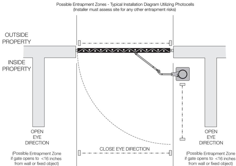
Figure 26 - GENERAL GATE LAYOUT WITH PHOTO EYES
