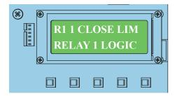
An example of a user relay function is shown here. Setting R1 to 1 creates an interlock signal to another operator's interlock input. The relay is released when the fully-closed limit switch is tripped (indicates that the gate is secure). Any open command energizes the relay.
