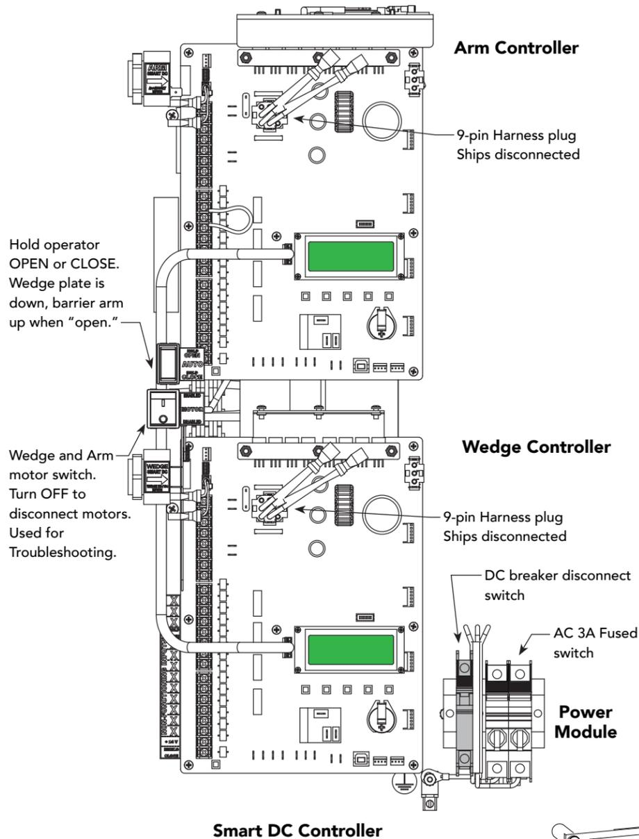
RED "Heart Beat" indicates Controller is receiving power. Flashing indicates AC or DC present. When AC power is lost, rate of RED blinking LED slows down.
