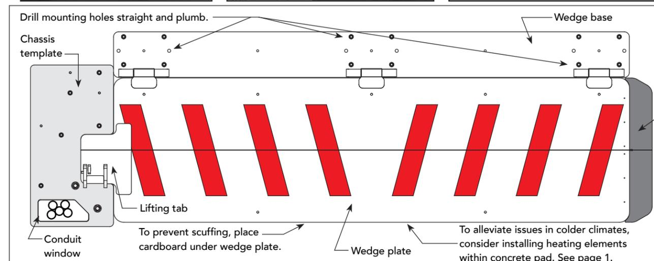
Install cover guard before securing the wedge plate to the concrete pad.
