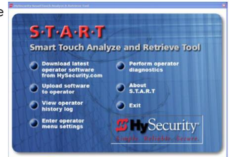
With S.T.A.R.T. software loaded on your laptop computer, you have an invaluable management tool for all HySecurity operators. The RS-232 serial port (found on the Smart Touch Controller), allows you to download system diagnostics and upload system configurations using the S.T.A.R.T. software. The free S.T.A.R.T. software is conveniently located at [www.hysecurity.com](http://www.hysecurity.com). Instructions for downloading S.T.A.R.T. are on the website.
