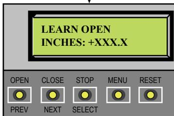
Hold the OPEN button until the gate slides to full open. Release the OPEN button. Note that if you go too far, you can press CLOSE to reverse direction. Press STOP twice to preserve the open stop location in memory.
