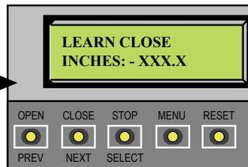
Hold the CLOSE button until the gate slides to full close. Release the CLOSE button and press STOP twice. The full close stop is retained in memory.
