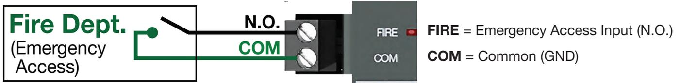
The fire input is meant to allow emergency personnel the ability to open the gate in an emergency situation without needing assistance. See **Emergency Gate Access**, below, for more information.
