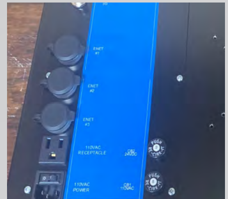
Back side of the HMI with connectors
