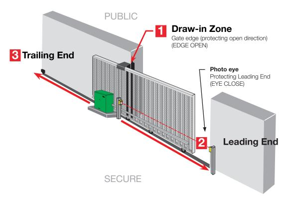
Installers must assess each specific site and install sensors that protect all potential entrapment zones.
