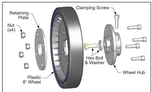
Figure 1: OLD 8" AdvancedDrive Wheel Dis-Assembly
