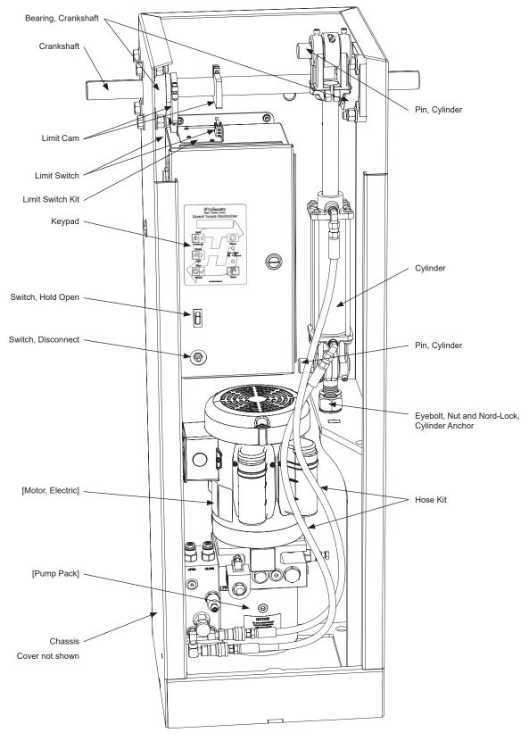
This drawing is a representation and should be used for parts reference only.
