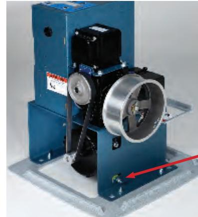
3. If tension is out of range, adjust the nut at the front base of the machine. Tightening nut increases tension.
