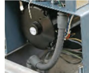
3. Feed AC wires through conduit into wiring panel. Secure to chassis.
