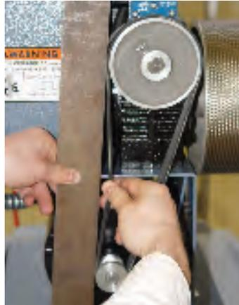
2. Place a straight edge on the belt long enough to span both pulleys. Pull the belt with two fingers from the middle of the span. The belt should deflect no less than 1/2" nor more than 5/8".
