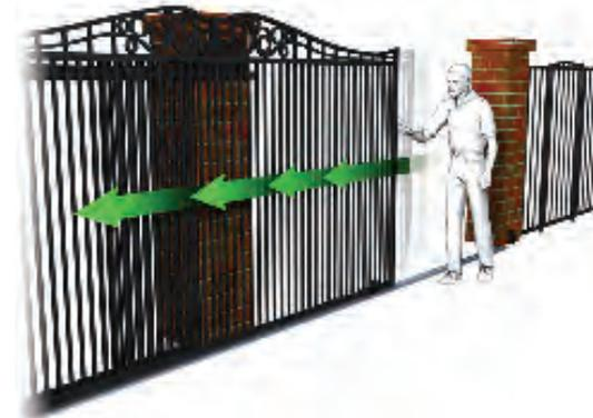
**Gate Speed Must Meet UL Speed Restriction**
