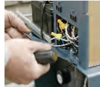
5. Secure wiring box with cover plate.
