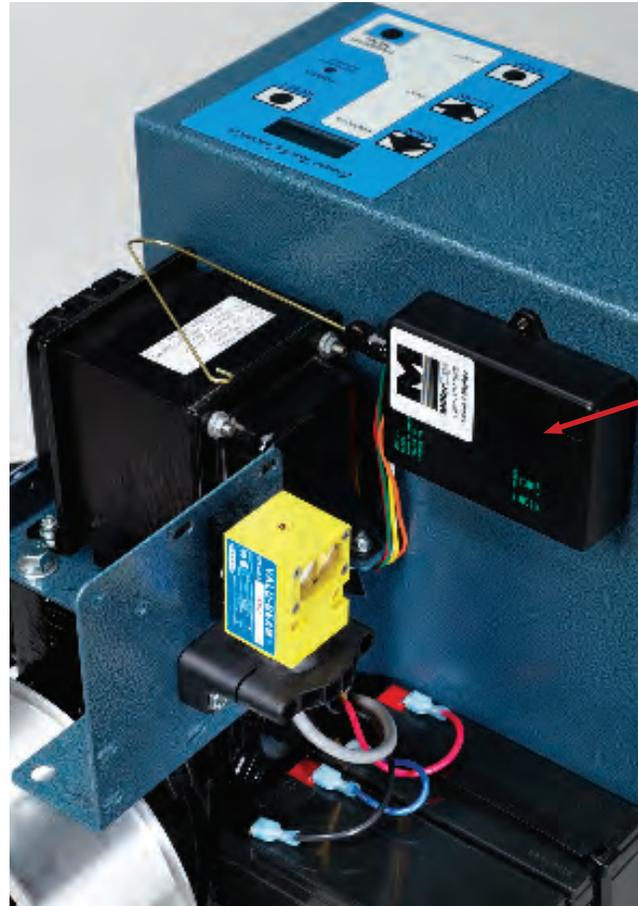
Radio receiver mounted on back of chassis using pre-drilled hole(s) (do not drill through chassis)
