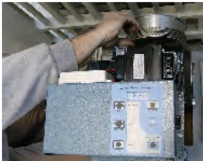
**5b.** To keep cable wound tightly together, stop winding and manually push the wraps together several times. SlideWinder 24 drum pictured in this and previous photos.
