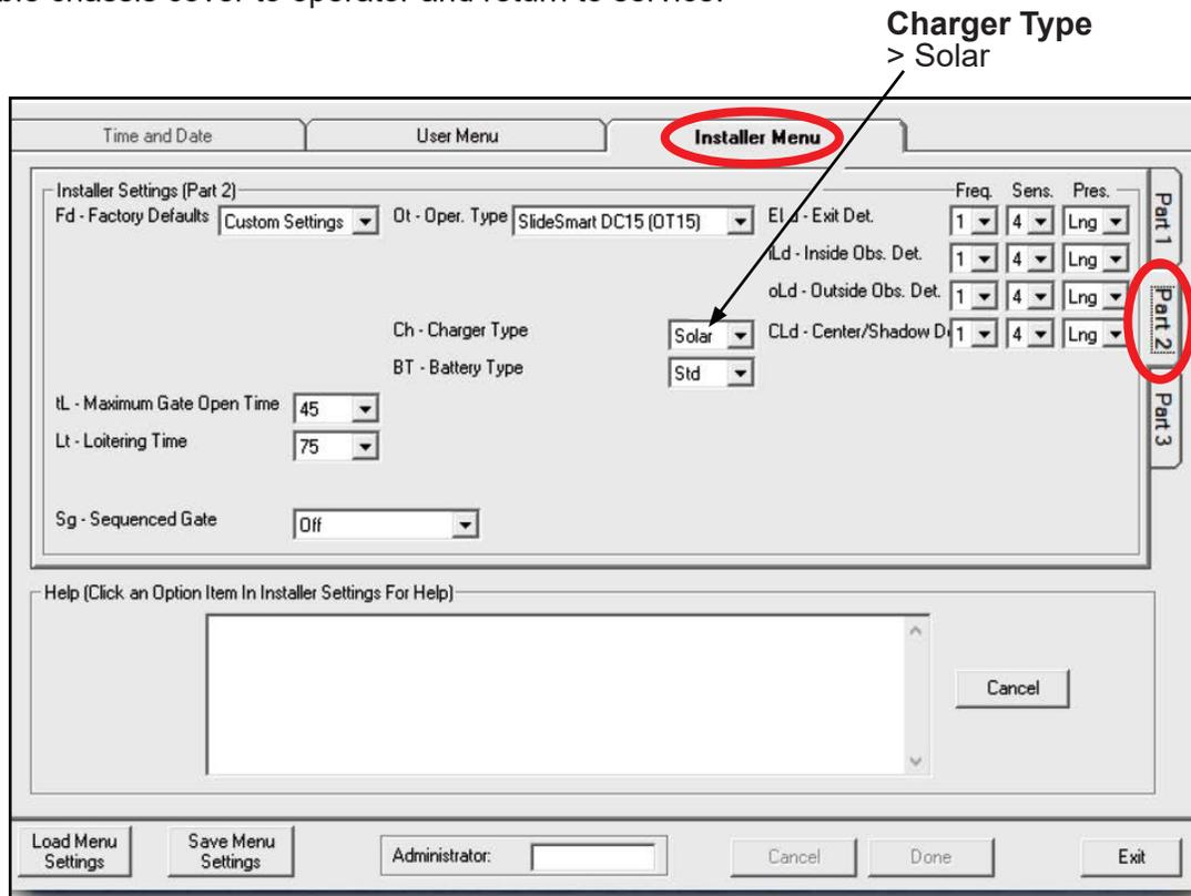
**FIG-8: START Software - Installation Menu Power Settings**
