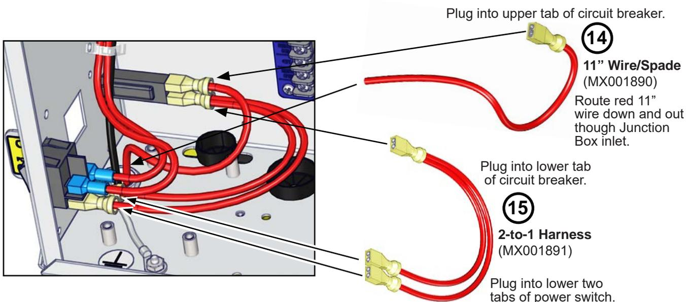
**FIG-5B: Installing Other Harnesses to Power Components**
