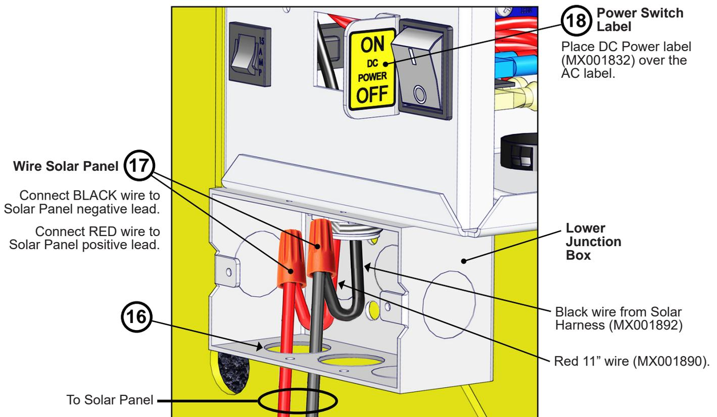
**FIG-6: Connecting Solar Panel Cable Leads**
