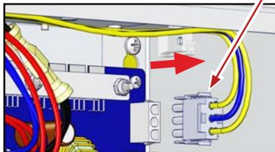
**FIG-3: Removing AC Transformer Harness**
