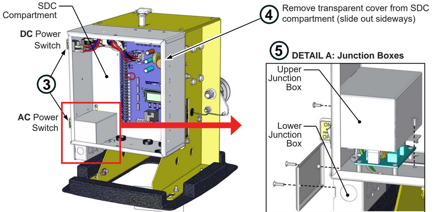
**FIG-1: Accessing Power Components and Wiring (Chassis Cover Removed)**
