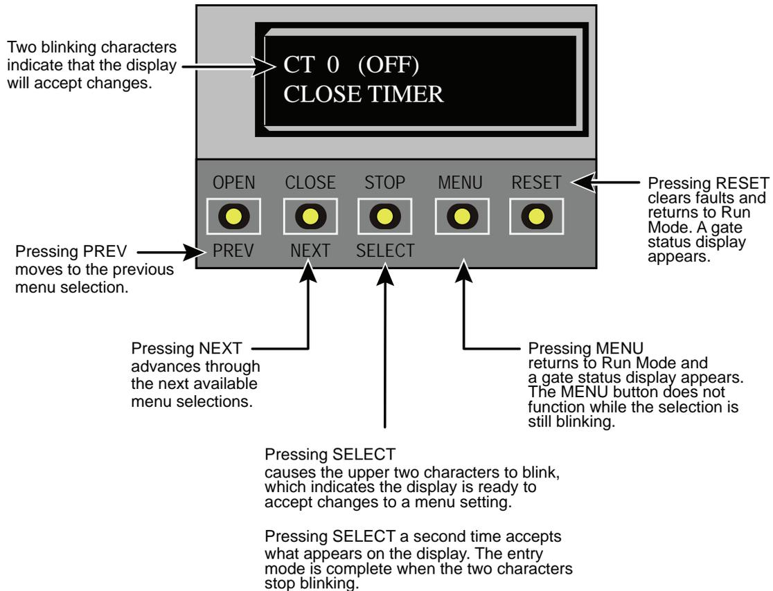
**FIG-7: SmartTOUCH Controller: Buttons and Menu Operation**
